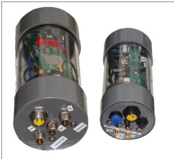
The WaterWiSe@SG sensor node processing unit features water-resistant packaging to allow use inside an access point if required. The 2009 version (left) is 120 x 260 mm in size, whereas the 2010 version (right) is 90 x 200 mm in size.
